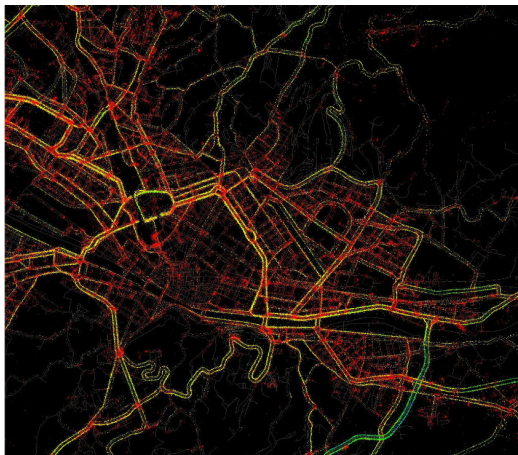
FIG 1. Aggregated GPS position data in the Florence area recorded during March 2008; the red dots corresponds to a recorded instantaneous velocity \leq 30 Km/h, whereas the yellow dots correspond to velocities in the interval 30 < v < 60 Km/h and the green dots to a velocity \geq 60 km/h.
