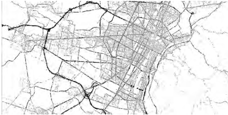
Figure 1 Torino, September 2007, 5 million GPS data corresponding to 800 thousands trajectories and 16 thousands vehicles on an area of 27 \times 23 km. Data provided by Octotelematics Spa.
